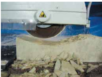
Sequence of a shape processed with vertical disc Sagomatura con disco verticale
